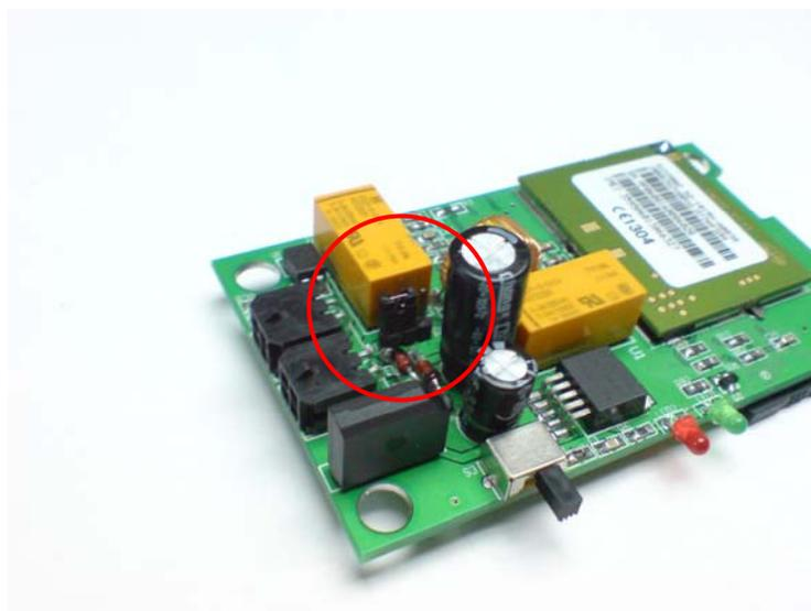
*Note: Relay 2 will supply DC voltage only according to the output DC voltage of adapter used. When 24VAC adapter is used, the voltage supplied would be 33VDC.*
